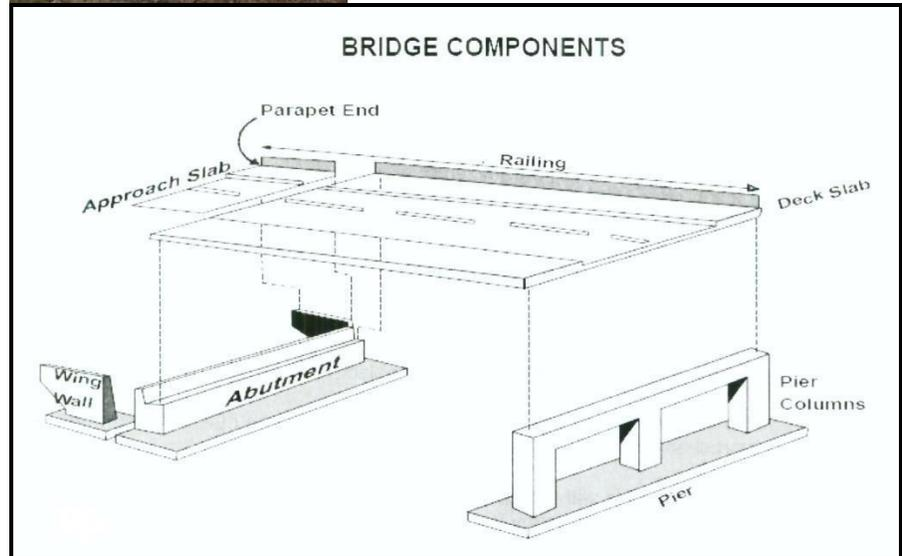
38. **Bridge Rail** - A [bridge parapet](#) or a barrier attached to a bridge deck to restrain motor vehicles, pedestrians, or other users. This includes guardrails which serve as bridge rails.
